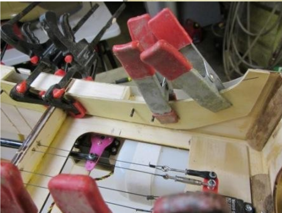
Using the wing rib as a pattern I had to make some plywood formers and glue them to the existing fuselage formers after ensuring that I hadn't changed the wing incidence and that I had repositioned the wing to align with the fuselage underside. These formers will have the Proskin fillet base glued to them.
