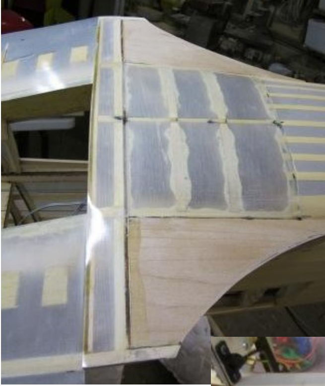
This is a picture of the completed underside infill and ply fillet supports.
